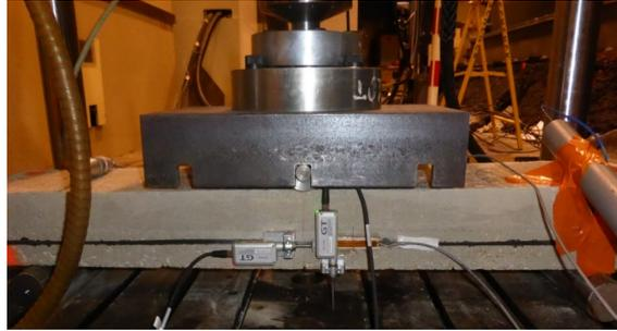
**Figure 3: 3-points bending set-up with the LVDTs and strain gauge sensors visible.**
