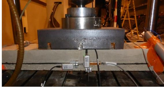
**Figure 3: 3-points bending set-up with the LVDTs and strain gauge sensors visible.**
